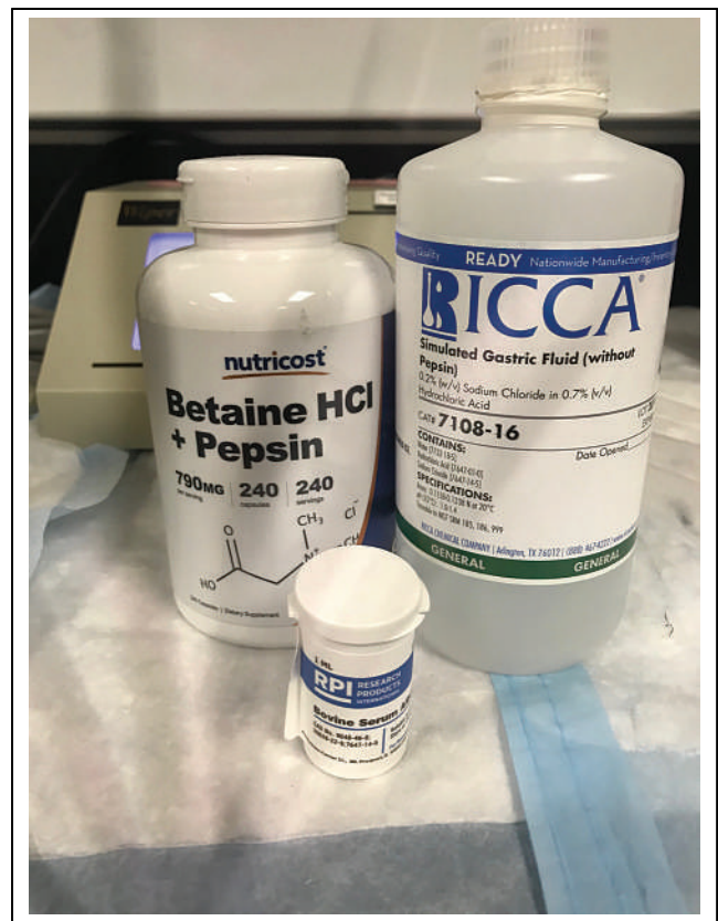
FIGURE 1. Materials used to simulate gastric environment and examine radiolabeling: simulated gastric fluid with HCl and pepsin. Bovine serum albumin was used to evaluate radiolabeling efficacy.
