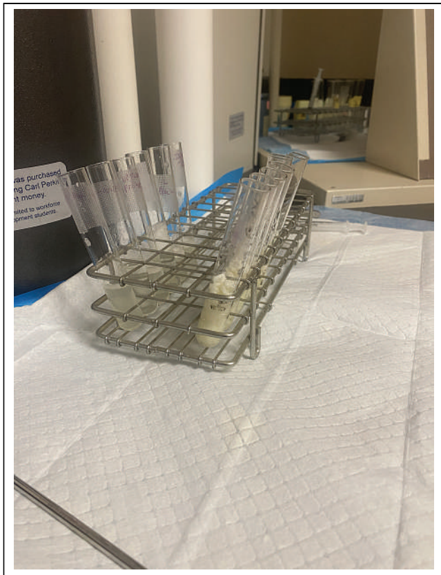
FIGURE 2. Twelve test tubes with radiolabeled cooked egg whites separated from simulated gastric fluid.
